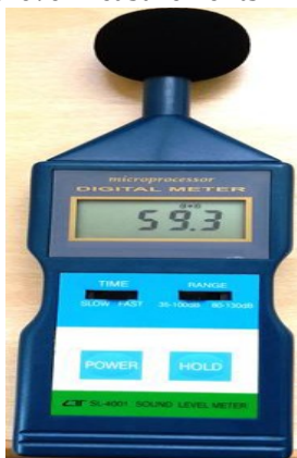
Figure 1: microprocessor based digital sound level meter ( SL – 4001)
